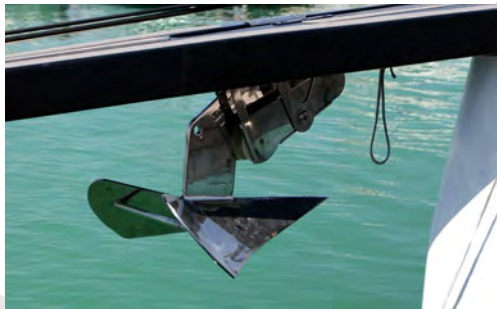
Carbon fiber bowsprit with integrated anchor support
