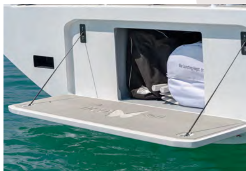
Liferafts locker accessible from outside
