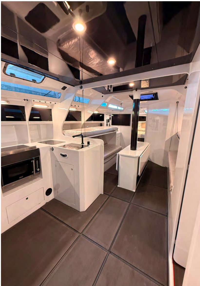
Carbon composite floorboards with EVA brushed cover
