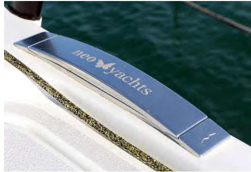
Retractable light aluminium custom bitts
