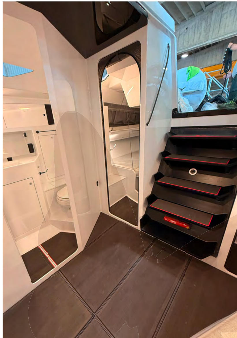
Carbon composite floorboards with EVA brushed cover
