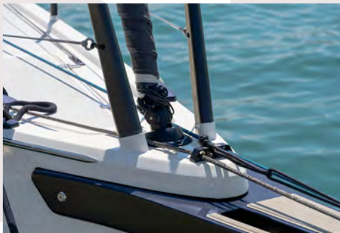
Carbon fiber pulpit and stanchions
