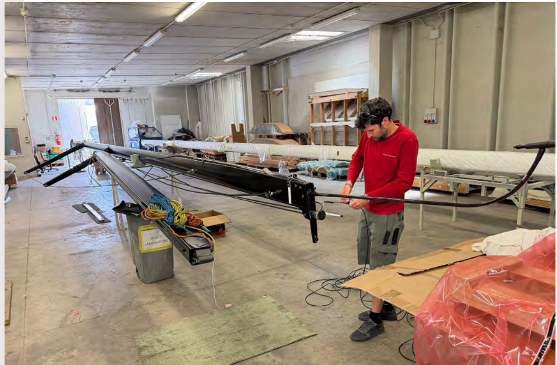
Carbon Mast and Boom with Carbon Standing rigging (optional)
